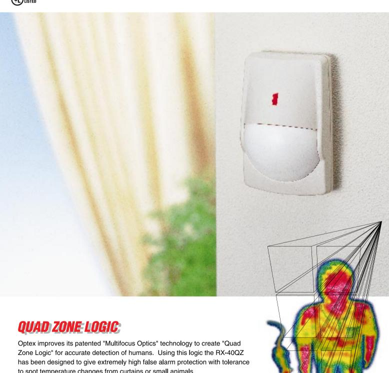
to spot temperature changes from curtains or small animals. Optex's Optical Quad Technology uses taller detection zones divided into upper and lower areas. It detects IR energy changes in both areas and then couples them for extremely accurate detections, offering very high reliability in
